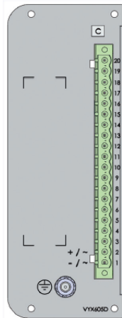
Figure 205 - Example of supply voltage card Power C 110-240
