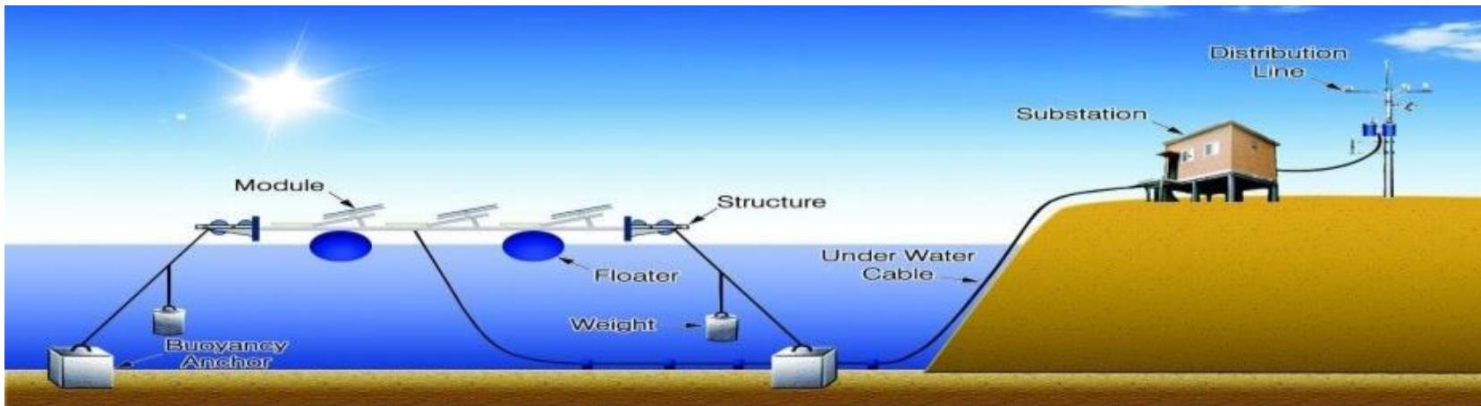
Basically, a floating photovoltaic plant consists of:
