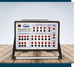
Electromechanical relays tests (550 VA available);
